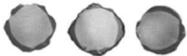
Figure 2: Defective CSPD observed in several 8 and 12 mm rebars.
